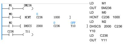
1. When M0 is ON, C236 will count in the interrupt mode when X0 changes from OFF to ON (see *错误! 未找到引用源。错误! 未找到引用源。* for the description of the X0 input frequency). When C236 changes from 999 to 1000, the C236 contact will be set. When C236 changes from 1001 to 1000, the C236 contact will be reset. When the C236 contact drives Y11, the execution of Y11 is determined by the user program scan cycle.
