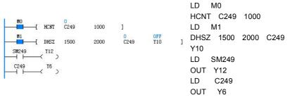
1. When M0 and X6 are both ON, C249 will count up when X0 changes from OFF to ON, or count down when X1 changes from OFF to ON. When C249 changes from 999 to 1000, the C249 contact will be set; when C249 changes from 1001 to 1000, the C249 contact will be reset. When C249 contact drives Y6, the execution of Y6 will be determined by the user program scan cycle.
