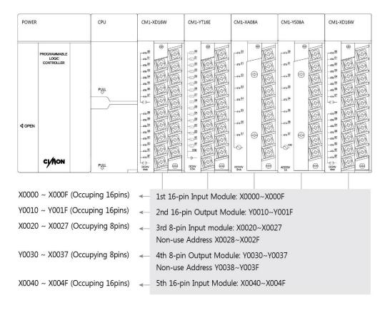
[Figure 15] Example of CM1-Series Module Composition (8-pin I/O Module)
