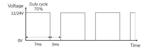
[Figure 7] Example of duty cycle control (PWM)
