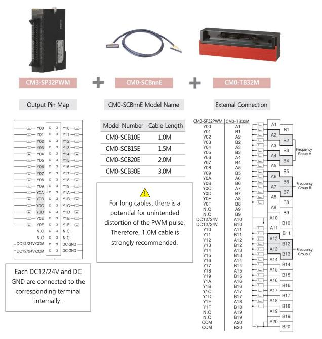
[Figure 4] Arrangement of terminals and its notations
