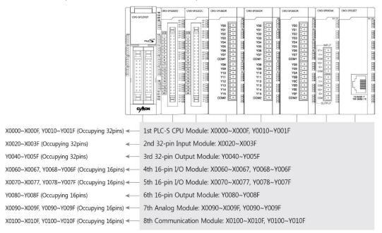
[Figure 18] Example of PLC-S Series Module composition
