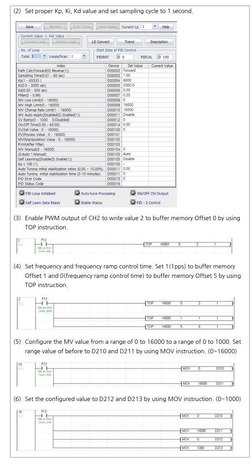
(7) Scale transform the MV value (D102) by using SCL instruction and save the value to D200.
