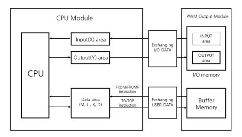
[Figure 5] Data exchange between PWM module and CPU
