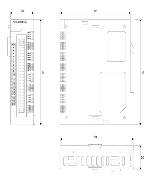
[Figure 3] PWM module appearance
