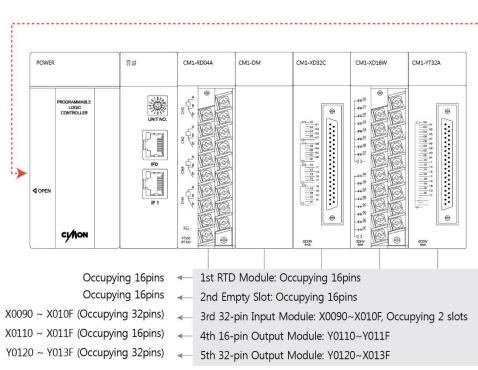
[Figure 17] Case of Additional CM1-Series Connection
