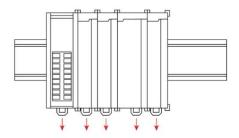
1. To unlock the module, pull Din Rail Locks positioned underside of each module.
