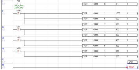
(1) Use TOP instruction to enter value 2 on buffer memory Offset 0 to enable channel PWM output.
