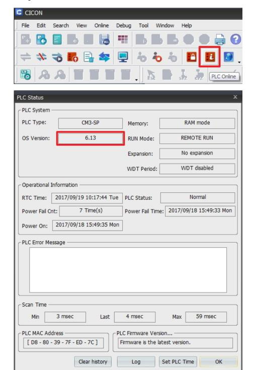
[Figure 2] Route to check CPU firmware
