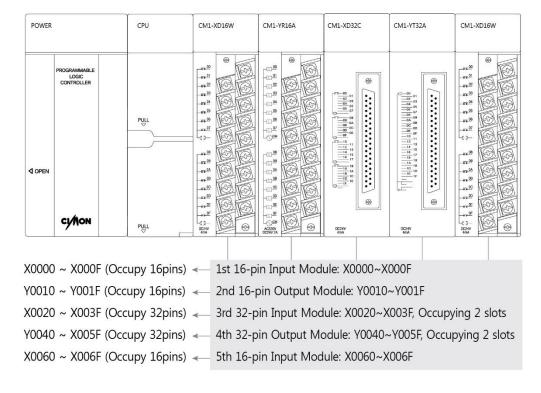
[Figure 16] Example of CM1-Series Module Composition (32-pin I/O Module)
