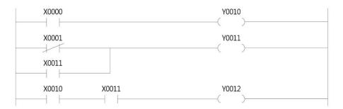
[Figure 19] Example of I/O configuration.
