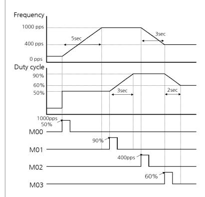
When M00 turns on, the system operates below:
