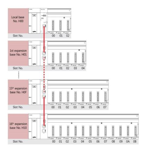
[Figure 10] Example of PLC-CM1 Series module extension
