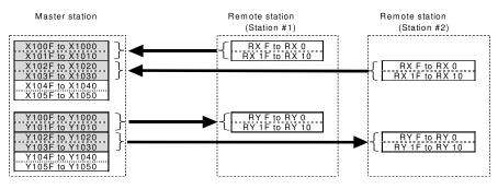
Figure 10.2 Relationship between Master Station Devices and Remote I/Os
