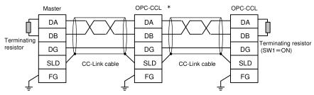
\* On CC-Link communications cards connected in the middle of the network, set their terminating resistor switches (SW1) to OFF (No insertion of terminating resistor).
