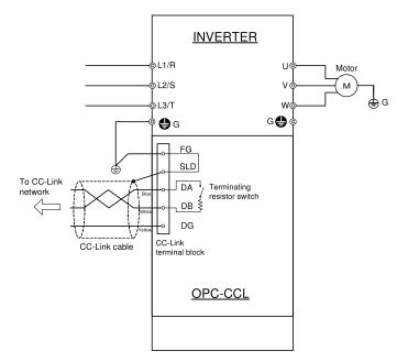
Figure 4.1 Basic Connection Diagram
