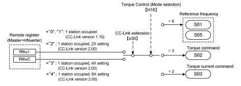
Figure 7.1 Torque control with RWw1 or RWwC
