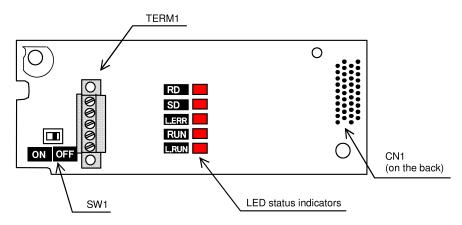
Figure 2.1 External View and Component Names
