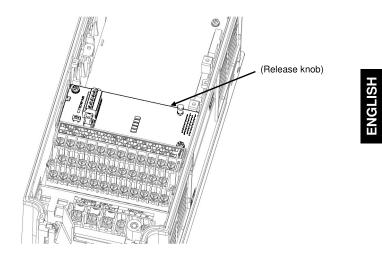
Figure 3.2 Mounting Completed (to FRENIC-MEGA A-port)
