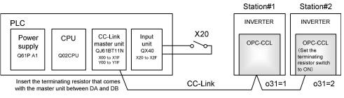
Figure 10.1 System Configuration
