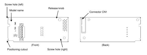
Figure 1.1 Names of Parts on CC-Link Communications Card
