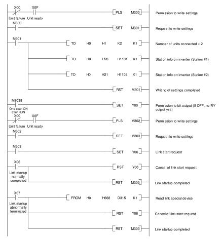
Figure 10.4 CC-Link Startup Program Example (for ACPU only)
