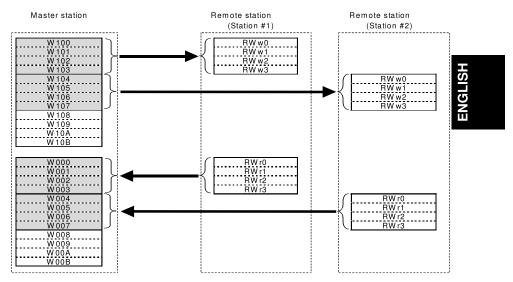
Figure 10.3 Relationship between Master Station Devices and Remote Registers
