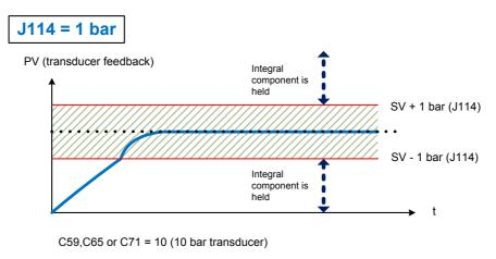
Figure 6.4: PID behaviour when function J114 is used.
