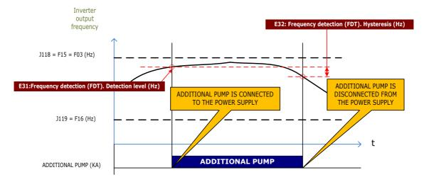
Figure 2.2: Additional pump's connection/disconnection time diagram
