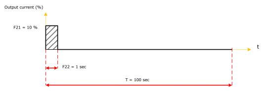
Figure 3.3: Output current when Dew Condensation prevention function is enabled
