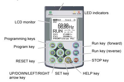
Figure 8.1: Names and Functions of Keypad Components
