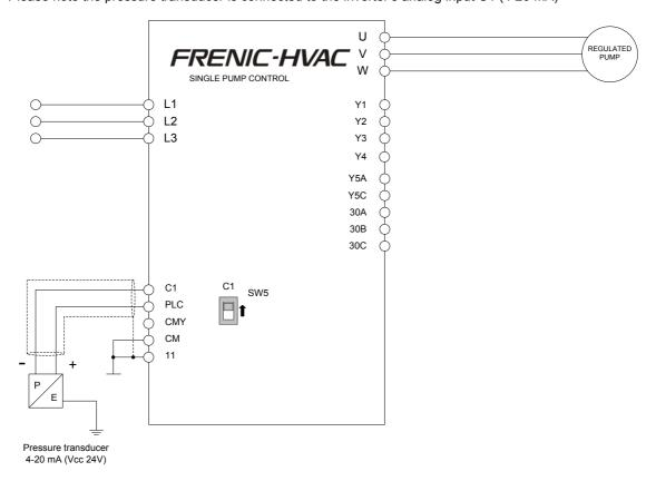
Figure 1.1: control schematic for a single pump
