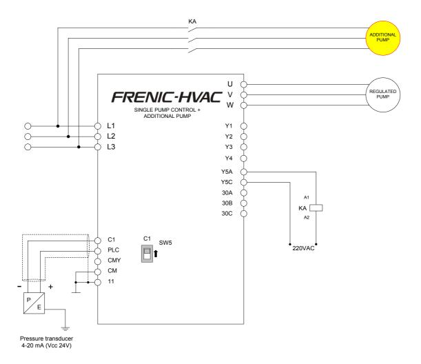
Figure 2.1: Schematic for single pump control with 1 regulated pump + 1 additional pump
