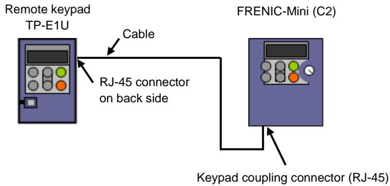
Figure 1-12 Connection Diagram between the TP-E1U and the FRENIC-Mini (C2)
