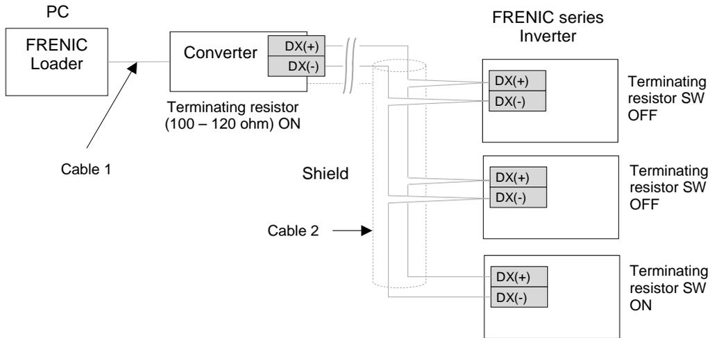
Figure 1-3 RS-485 Connection Diagram (Terminal Block Connection)
