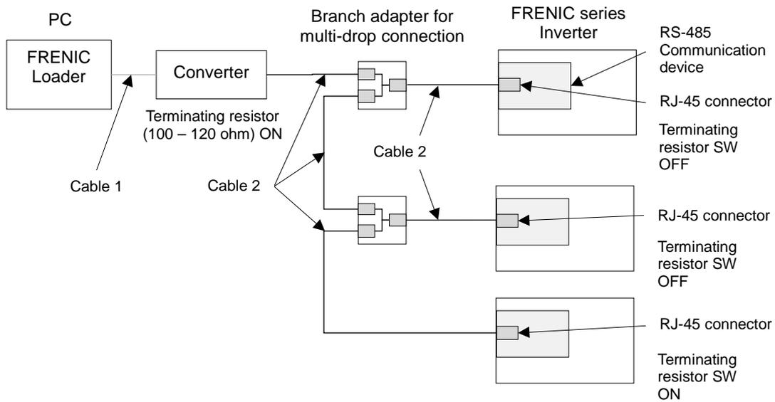
Figure 1-2 RS-485 Connection Diagram (RJ-45 connector Connection)
