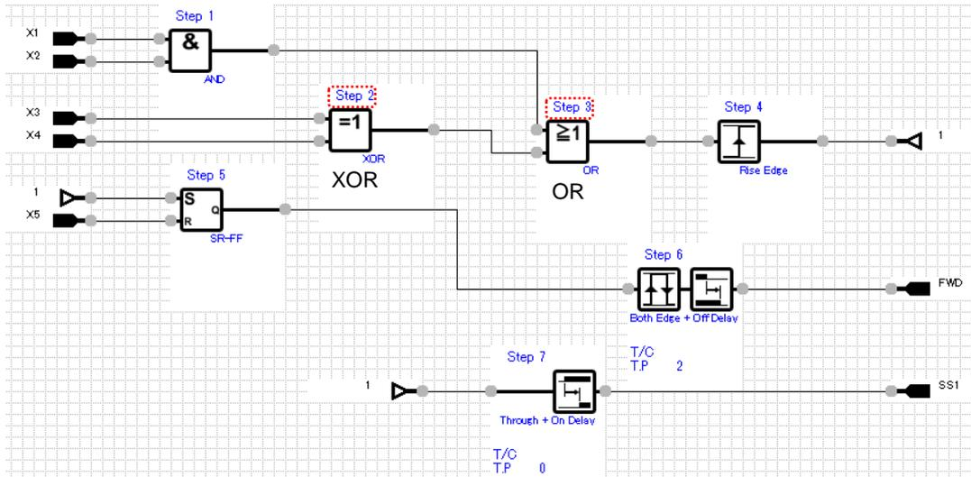
Now the XOR circuit and the OR circuit are assigned Step 2 and Step 3, respectively. This means that the output of the XOR circuit is input to the OR circuit in the same execution cycle as the OR circuit.
