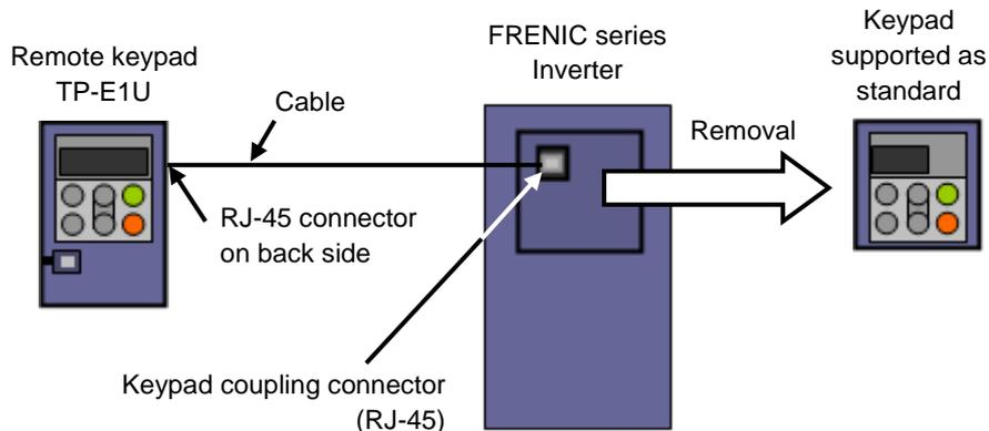
Figure 1-11 Connection Diagram between the TP-E1U and the Inverter (Other than the C2 Model) (Connection Using a Communication Cable)
