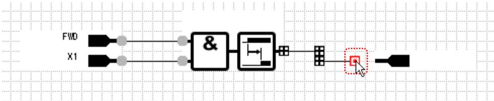
Once the connection line is connected to the symbol, the square at one end of the connection line changes from red to black.
