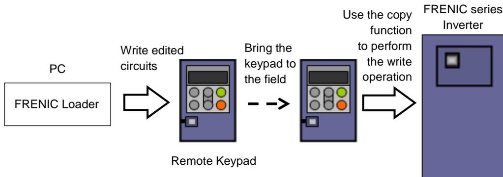
Figure 2-1 Workflow of writing circuits to a keypad
