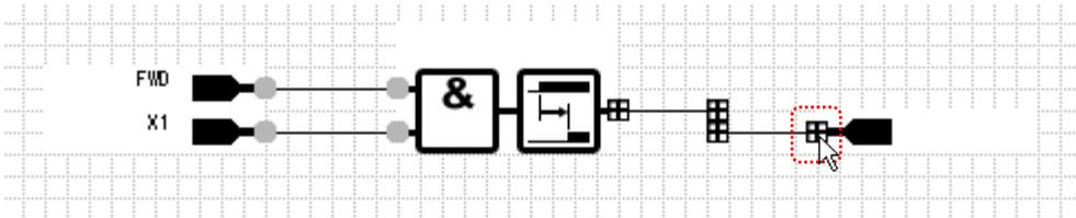
When you release the left mouse button, the square at one end of the connection line changes from a black square to a gray circle, indicating that the connection line is complete.
