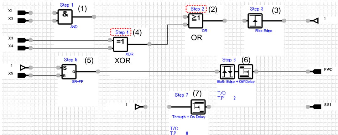
In the above example, the XOR circuit is assigned Step 4, and the OR circuit Step 2. As the result, the output of Step 4 is connected to the input of Step 2
