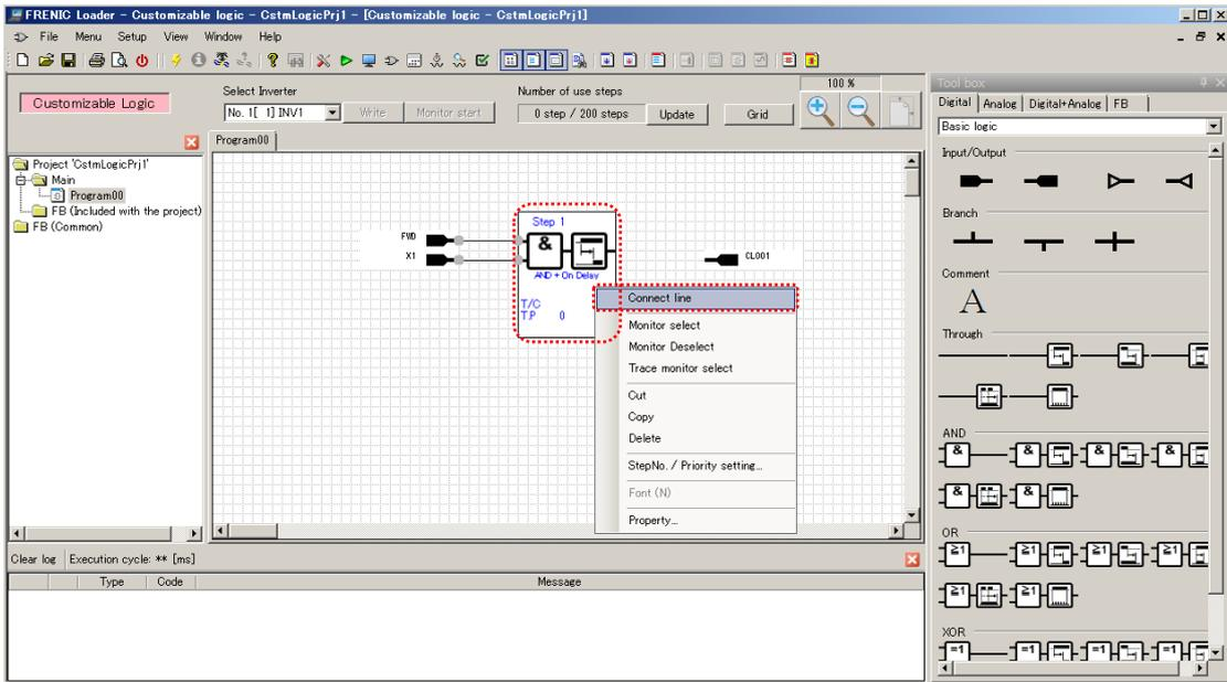
The connection line appears. Hover the mouse pointer on the red square at one end of the connection line and move it to the symbol you want to connect while holding down the left mouse button.
