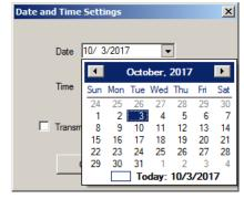
\* Clear (remove from) the [Transmit the same date and time as OS] check box to send your specified date and time. Click [OK] to send the date and time to the inverter.
