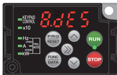
Figure 4.3-1 Display of the LED Monitor after Power-on
